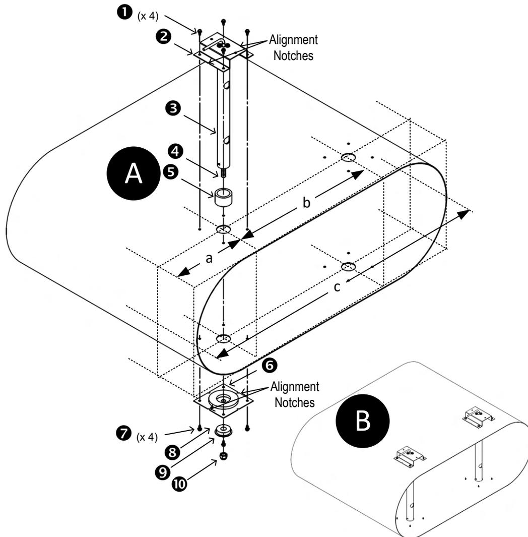
Step 1. Select a location in the duct or plenum opening that meets or exceeds EBTRON's recommended placement guidelines.
