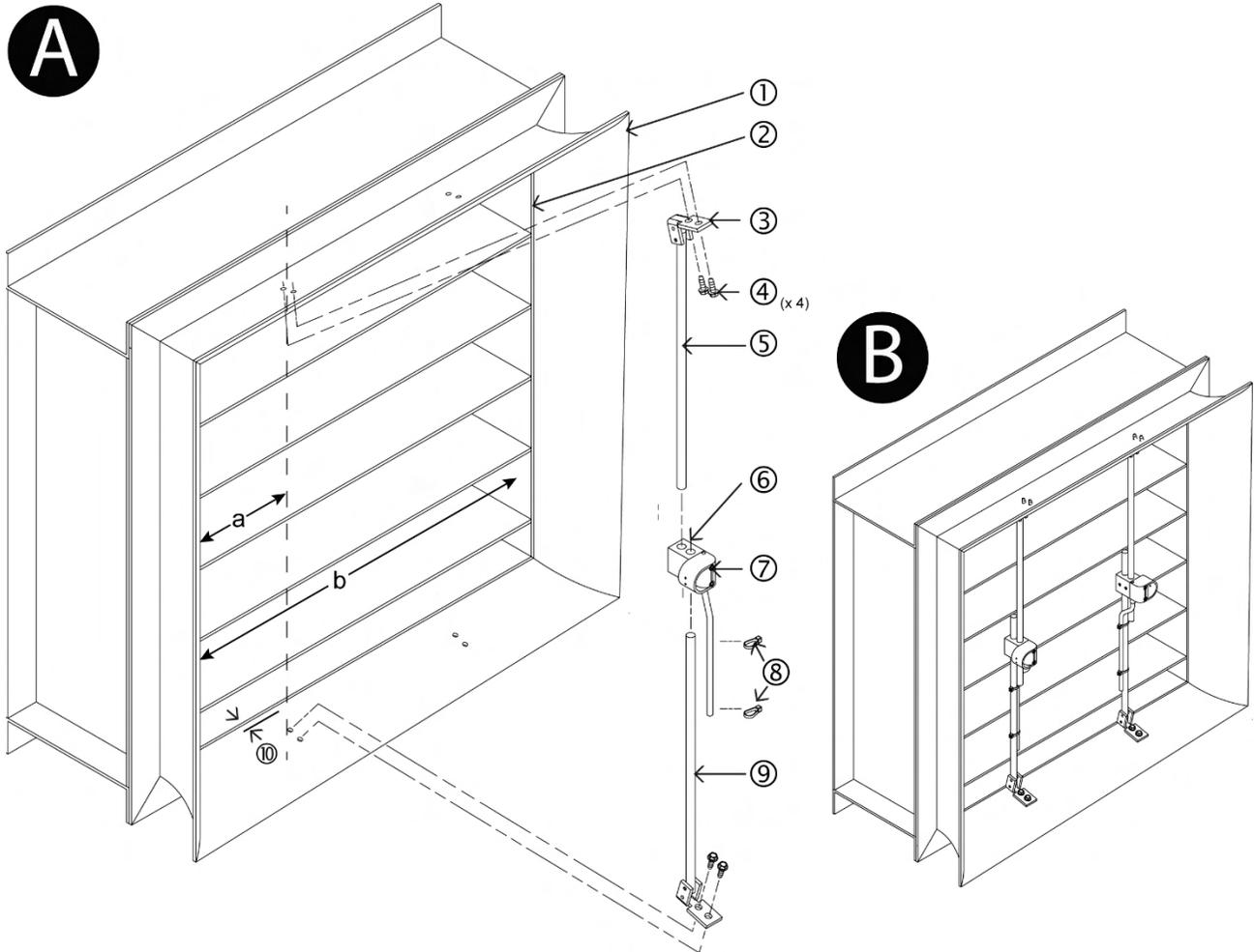
Step 1. Select a location on the damper flare that allows clearance for probe placement and installation.
