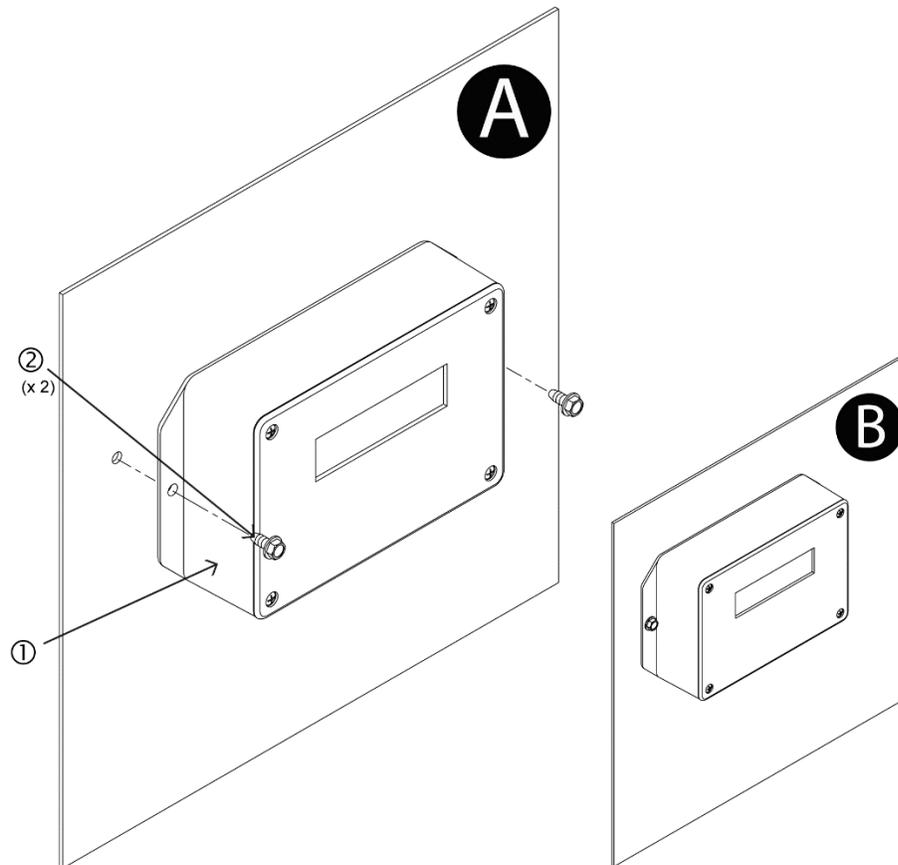
Step 1. Locate a position for the transmitter so that the connecting cables from all of the sensor probes will reach the receptacles on the bottom of the transmitter enclosure.
