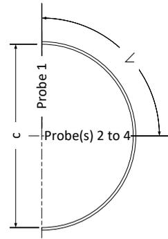
**i** *If the probes were ordered for a duct with internal insulation, use the external diameter of the duct for 'c' to calculate 'b'.*
