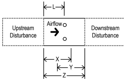
“Z” is Less Than X+Y (CCOAI Louver and Straight-through Hood Applications)
