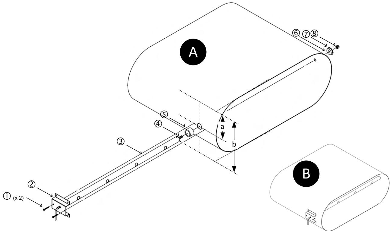
Step 1. Select a location in the duct or plenum opening that meets or exceeds EBTRON's recommended placement guidelines.
