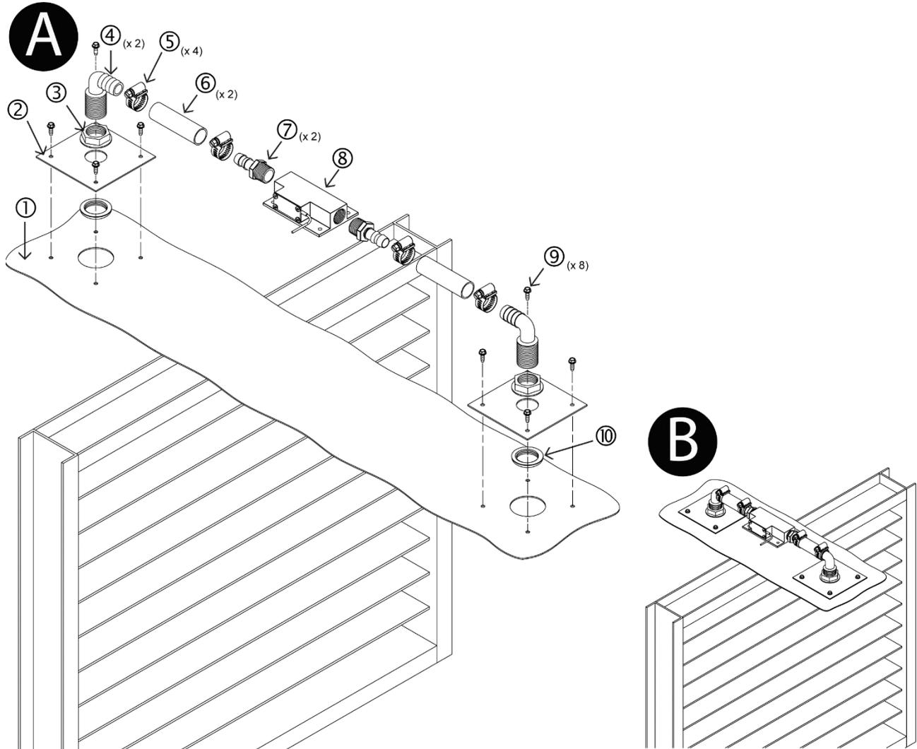
Step 1. Select a location along the duct on both the upstream and downstream side of the damper that allows for the bleed sensor placement and installation.
