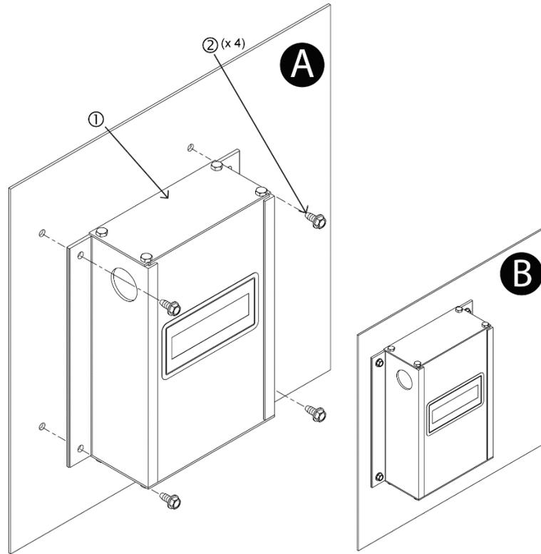
Step 1. Locate a position for the transmitter so that the connecting cables from all of the sensor probes will reach the receptacles on the bottom of the transmitter enclosure.
