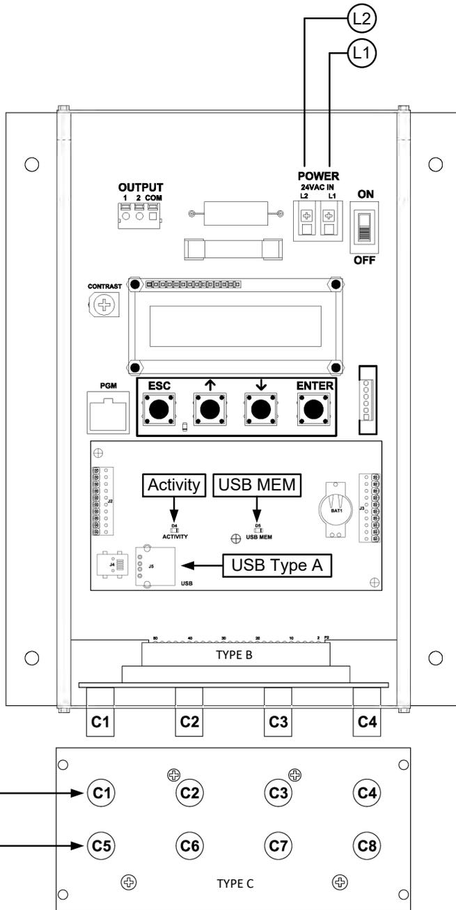
8. Transmitters with a USB data logger log the average airflow, average temperature, individual sensor node airflow and the individual sensor node temperature at 5-minute intervals using Universal Time Coordinated (UTC) based on an onboard real-time clock, whenever power is applied to the transmitter. Data files are automatically appended on power-up. The time zone and interval can be modified by the user using EB-Link software.
