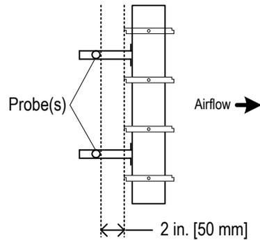
Step 13. Probe installation is complete! Figure “B” shows a completed two probe installation.
