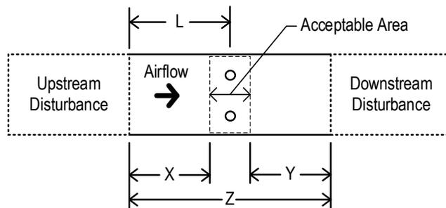
“Z” is Less Than X+Y (Ducted Applications Only)
